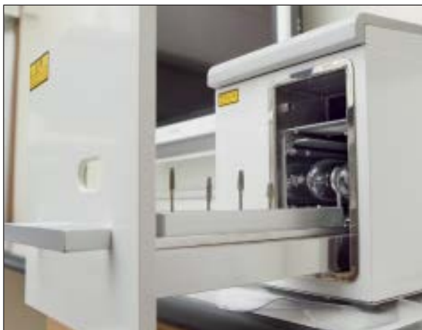
Fig 1a The photo device used for photofunctionalization of dental implants (TheraBeam Affiny). Implants are placed on a sliding stage. The device performs an automatic program of 15 minutes of UV exposure and 5 minutes of ventilation.
