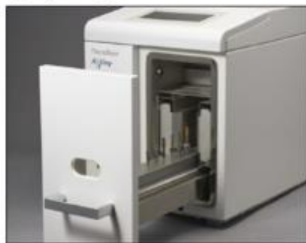
Figure 7b: A photo device used for photofunctionalization. The device provides an automatic 15- to 20-minute program of conditioning with optimized wavelength and strength of UV light treatment.
